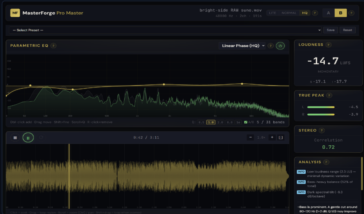
31-band parametric EQ with live spectrum, loudness metering, stereo correlation, and AI analysis.
